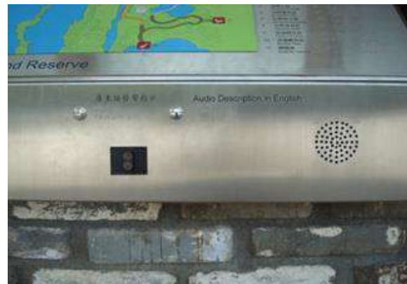
Figure 6-24: Speaker and buttons in talking signs
